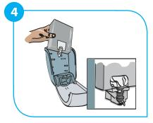
Fit cartridge into Soft Care dispenser unit ensuring the nozzle is in place.
