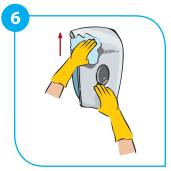
When cleaning the dispenser, support the front cover with your fingertips and wipe in vertical movements from the bottom to the top to prevent the product from being dispensed.
