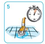
Agitate floor. Leave for 5 minutes. DO NOT allow floor to dry out.
