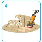
Allow to dry and then buff to a shine with a high speed rotary machine with a suitable grade pad or brush.
