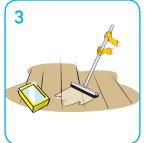
Using clean mop or applicator, apply seal. Work with the grain and avoid overlapping.
