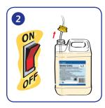
Switch off machine and wearing gloves and goggles remove feeder tube from empty container.
