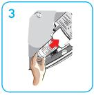
Insert tip of refill cartridge into nozzle inside the dispenser cover.
