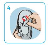
Slide base of refill cover into place slightly sideways, and twist refill to align it into slot.
