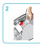
Lift (gently) the old cartridge upward and slide its base out first.
